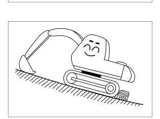
Avoid traveling in a cross direction on a slope as it can cause the danger of rolling over and sliding.
