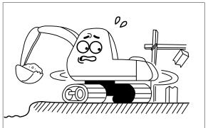
The operation on a slope is dangerous. Avoid operating the machine on a slope of over 10 degree.
